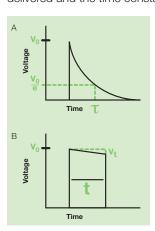
A, exponential decay pulse from a capacitance discharge system. When a capacitor, charged to an initial voltage  $V_0$ , is discharged into cells, the voltage applied to the cells decreases over time according to the equation  $V = V_0 e^{-\tau t/RC}$ , so that at time  $t = \tau$ , the voltage is  $V_0/e$  of the initial value.
